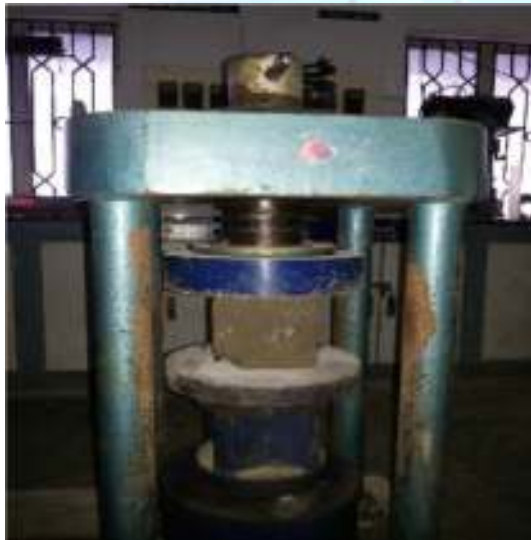
Fig 2. Testing of compressive strength of concrete.
